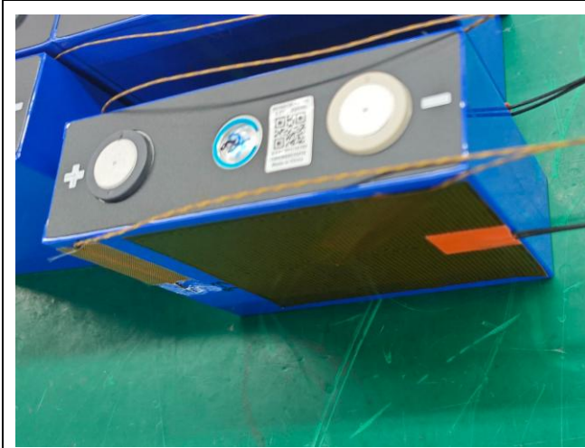
Figure 10 – Cell with heater. 1 piece of 152.4 mm by 203.2 mm for each wide surface, total 2 pieces for cell 9.
